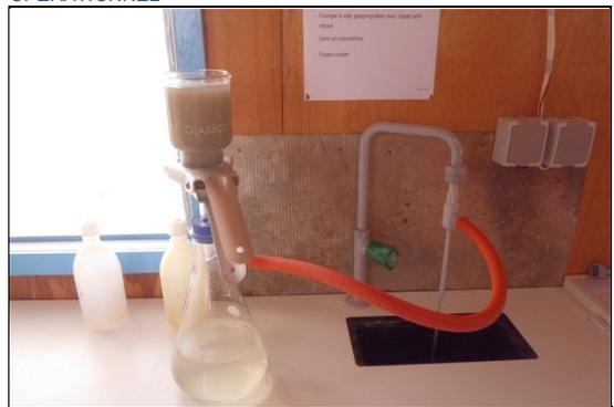
FILTRATION SOUS VIDE HYDRAULIQUE POUR LA MESURE DES MES
