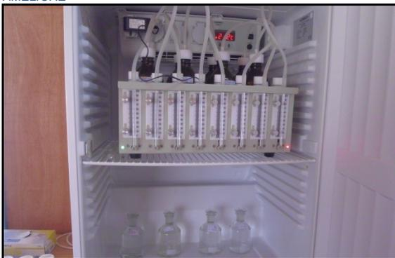
MESURE DE LA DBO5 AVEC OXYMETRE DE CWE DANS L'INCUBATEUR DU MOE
