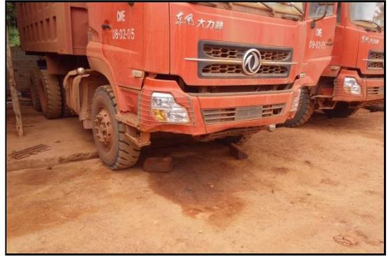
TRAVAUX REALISES EN DEHORS DE LA DALLE ET DU DRAINAGE AVEC POLLUTION DU SOL (GARAGE CONCASSEUR)
